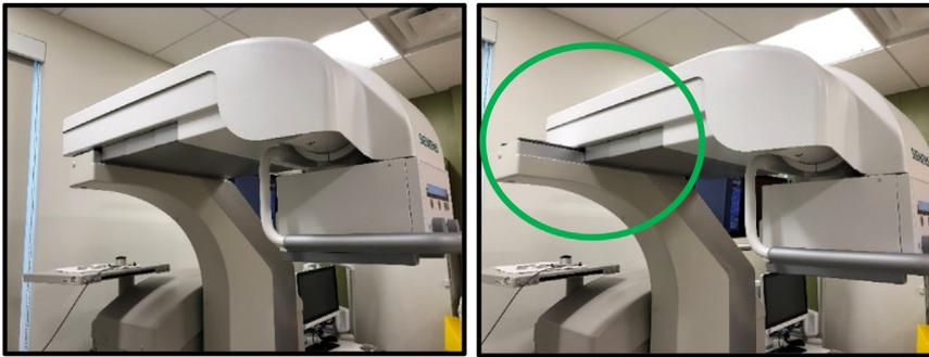
**FIGURE 24** Left: Longitudinal translation of the tube assembly is not aligned to the image receptor. Right: The alignment is centered with the image receptor, and the assembly is locked for imaging in fluoroscopy mode or radiography/acquisition mode, as required
