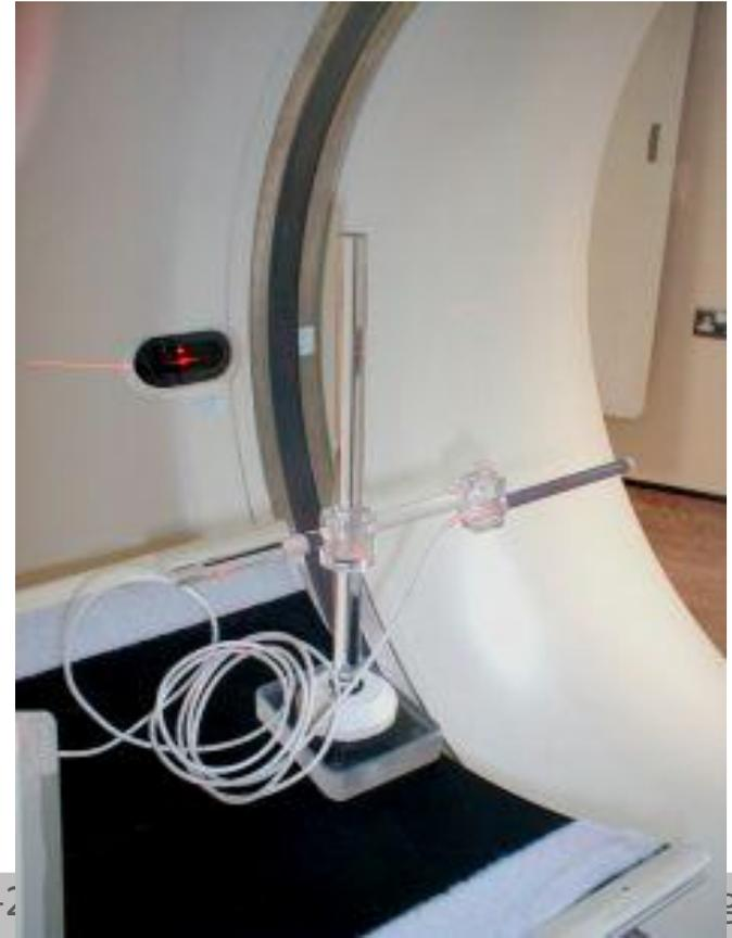
$C_{a,100}$  – CTDI measured in air, integrated over 100 mm, **mGy**
