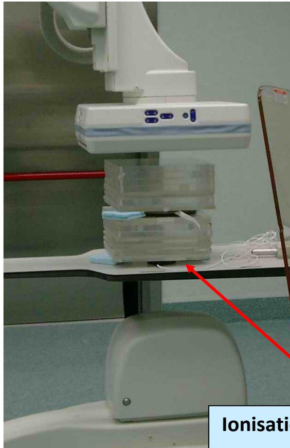
**Ionisation chamber to measure phantom entrance surface air kerma rate ( $K_e$ )**
